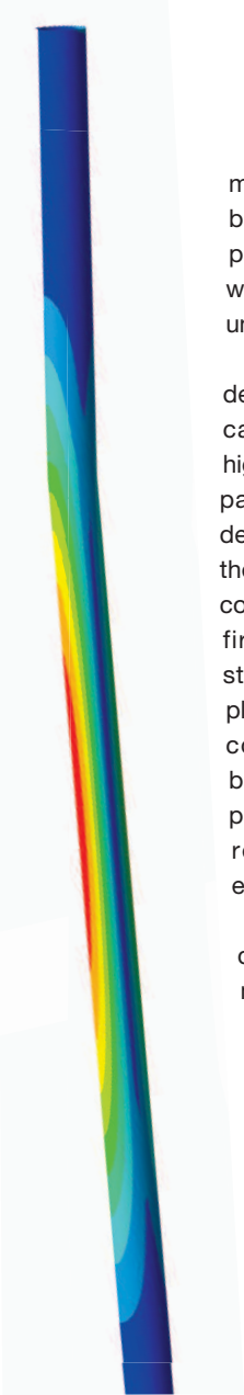
Nonlinear springs were used to represent soil forces acting on the conductor.
